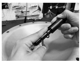
7. Tool is not required to install third O-ring. Pinch the O-ring between your index finger and thumb as shown, and insert into the remaining O-ring groove in the automatic valve.
