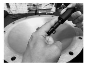
3. With your finger still covering the slide, use your other hand to push the slide forward to properly position the O-ring into the tool.
