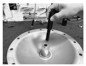
6. Re-insert O-ring tool slide into the body of the tool until O-ring grooves align. Position the second O-ring into the second groove as shown. Use your finger to cover top of slide to prevent O-ring from slipping out. Repeat steps 3 through 5 to install the second O-ring in the second groove.
