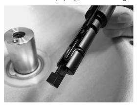
4. With the O-ring still positioned in the tool, insert entire tool into the automatic valve until the shoulder of the tool body is flush with the top of the automatic valve.
