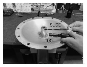
2. Position the first O-ring into the first groove as shown. Use your finger to cover top of slide to prevent O-ring from slipping out.
