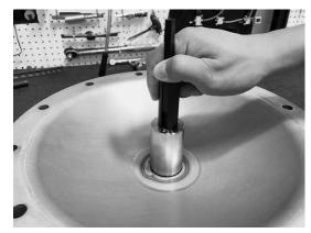
5. Hold down on the tool and carefully remove the insertion slide from tool body. Remove the tool from the automatic valve. The first O-ring should now be in place.
