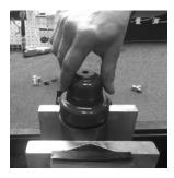
5. Insert new diaphragm O-ring ® into groove in spring housing ®. Press O-ring into groove to ensure it is fully seated.
