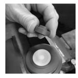
9. Remove assembly from vise. Remove diaphragm ⑤ from recess in body ④. If diaphragm is difficult to remove, invert body and insert a small blunt rod or tool in fluid port to push diaphragm from body. Take care not to damage diaphragm while removing. Inspect diaphragm and body for signs of chemical attack, wear or damage and replace as needed.
