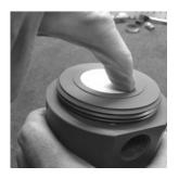
6. Insert spring seat <sup>®</sup> into recess in spring housing <sup>®</sup>, ensuring side with the longer pin will be facing spring <sup>⑦</sup>.
