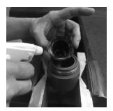
The bladder/bellows sealing ring is used to seal the body ④ and dampener housing ② together. Lubrication is critical so that the O-ring groove in each component will seat against the bladder/bellows sealing ring smoothly and without distortion.
