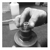
Use caution to ensure spring seat stays centered in spring housing recess during assembly. After tightening, remove assembly from vise and confirm spring seat is centered in spring housing recess by looking through threaded bore in spring housing.
