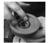
4. Insert new diaphragm ⑤ into recess on body ④ with conical protrusion inserted in the port in center of body. Run your fingers around diaphragm outer edge to ensure that it is fully seated in recess.
