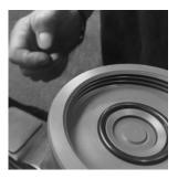
7. Place spring housing <sup>(9)</sup> in a vise with spring seat <sup>(8)</sup> facing up and clamp at flats with soft jaws or wooden blocks. Apply solution of soap and water as a lubricant to threads on spring housing and body <sup>(4)</sup>. Hand tighten spring housing and body together until snug. Use a spanner wrench or large adjustable pliers to tighten until lines marked before disassembly line up. Insert spring <sup>(7)</sup> into threaded bore of spring housing.
