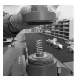
7. Remove diaphragm O-ring ® located in spring housing ® groove. Inspect O-ring for signs of chemical attack, wear or compression-set and replace as needed.
