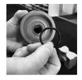
8. Using a large flat head screwdriver, remove adjustment screw ® from spring housing 9. Inspect adjustment screw and spring housing for signs of chemical attack, wear or damage. Pay particular attention to threads and replace parts as needed. Inspect spring ® and spring seat ® for signs of chemical attack, wear or damage and replace as needed. Note orientation of spring seat with regard to spring and diaphragm ®.
