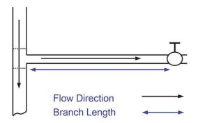
If water is flowing in the branch line and the valve is closed quickly, a shock wave will develop. Its inception follows the same sequence of events in our hypothetical example. One small difference is that some of the intensity of the waves will be lost in the "Tee" as it is open to the main pipeline on either side. Still, a significant portion will be reflected back toward the valve.
