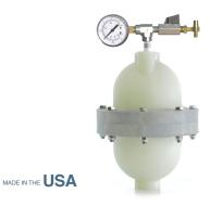
The J Model air control consists of a compound pressure gauge, a vacuum tight ball valve and a Venturi valve. Compressed air passing through the Venturi valve at high speeds creates a low pressure area. This evacuates air from the stabilizer to create an internal vacuum. Conversely, when the flow of air through the Venturi valve is diverted into the stabilizer, a pressure charge results in optimized pump efficiency and productivity.
